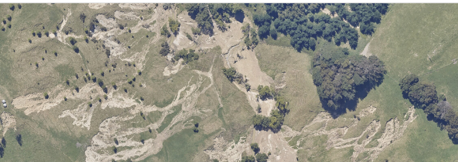
An aerial image of erosion and sedimentation caused by Cyclone Gabrielle in Hawkes Bay (selected from aerial data provided by LINZ Data Service). According to a Manaaki Whenua Landcare Research report, the reduction in landslide probability during Cyclone Gabrielle, in land clothed in woody vegetation, was substantial in Hawkes Bay through to Tairāwhiti, particularly where there was indigenous forest cover.
