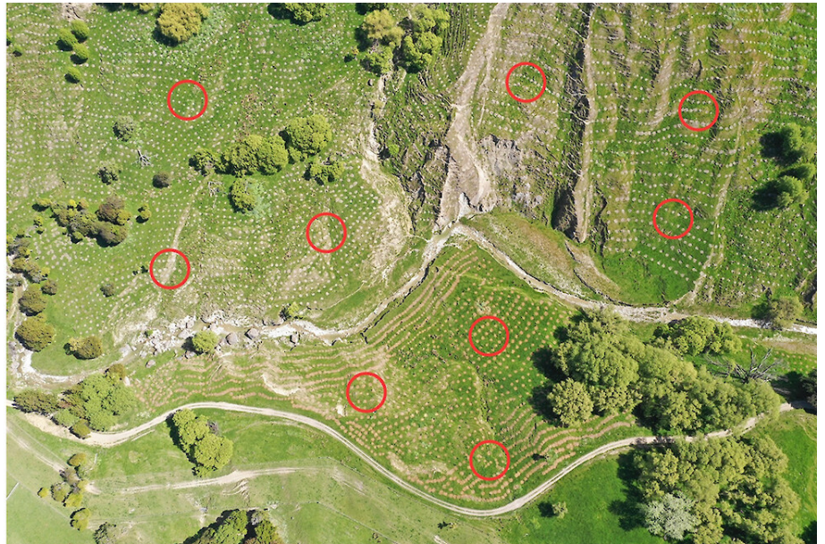
Figure 1: Ideally plots should be distributed evenly along a transect or in a grid pattern across the planting site to avoid sampling bias. However, in practice, a rigid grid of plots is often difficult to achieve with highly variable terrain and where placement of plots needs to avoid tracks and existing vegetation. The aim is to spread plots evenly across a representative area of the planting site as shown for this recently planted Hawkes Bay hill country station (right).
