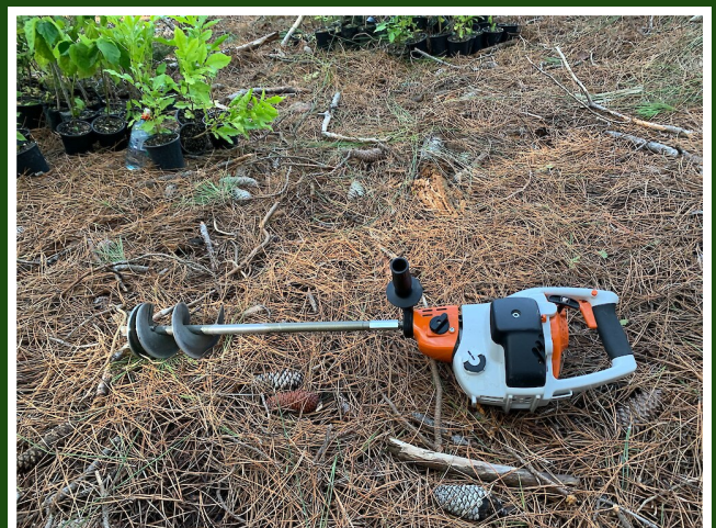
A petrol-powered motorised planting drill with light auger is an efficient way to provide planting holes, especially for community planting days to ensure consistent depth of planting.
